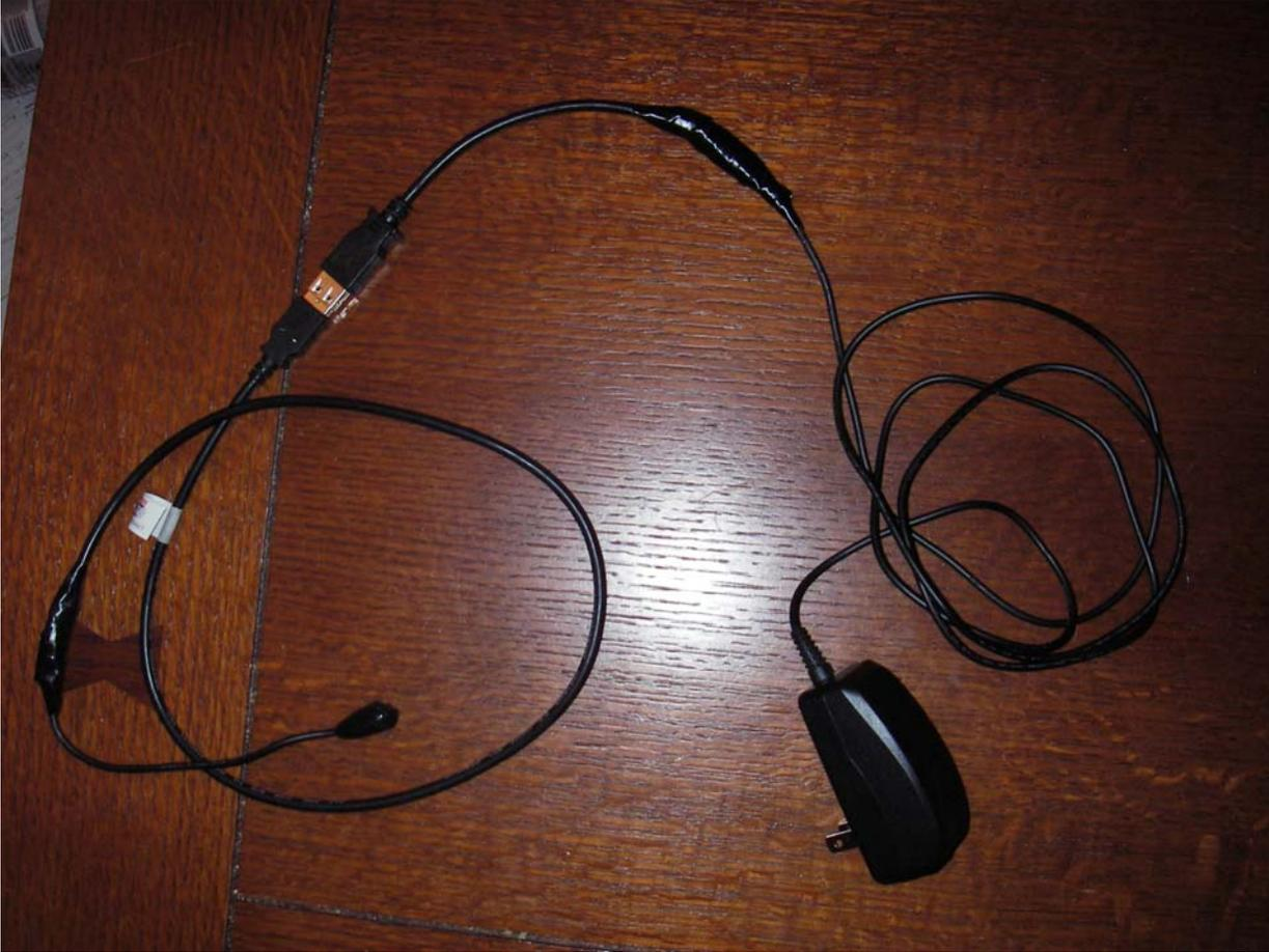
**You can now connect the AC adapter to your Zodiac using the USB connector, or use the USB cable to charge your Zodiac from various USB chargers/battery packs etc. such as those provided by [www.boxwave.com](http://www.boxwave.com)**
