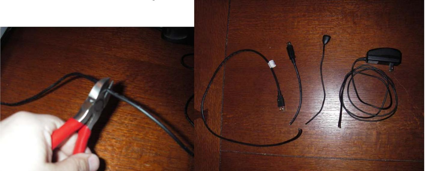
**Step 2:** Strip the outer layer of insulation from the two ends of the USB cables and from both ends of the Zodiac AC charger cables about 2 inches from the ends.
