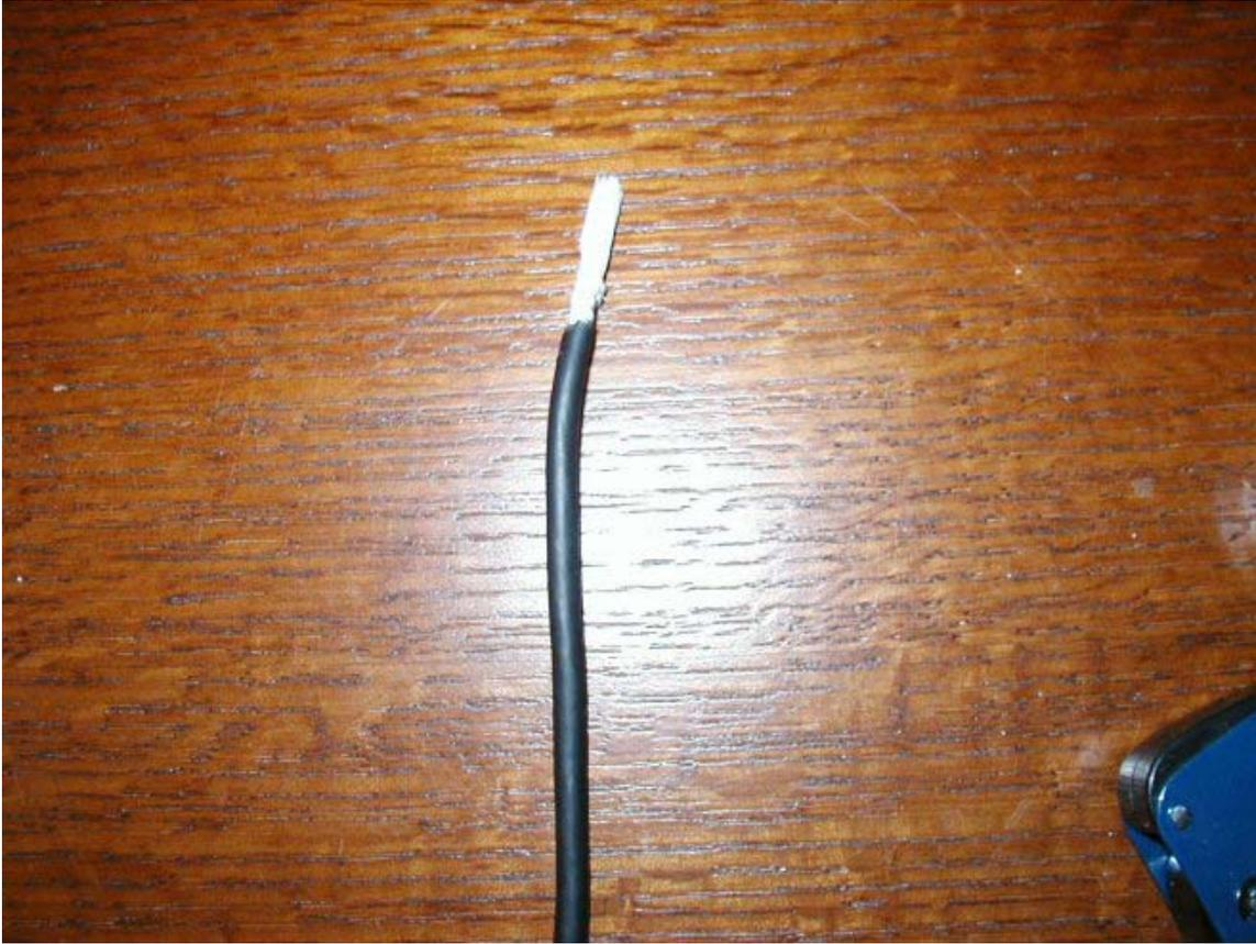
Step 2: Next remove and cut off the white paper stuff that surrounds the wires. The black and red wires exposed provide (+) and (-) voltage to the hotsync adapter. These are the ones you will splice to the car charger. Inside the wire mesh are the 4 wires from the USB connector. The wire mesh and foil protect the data in these cables from electrical interference.
