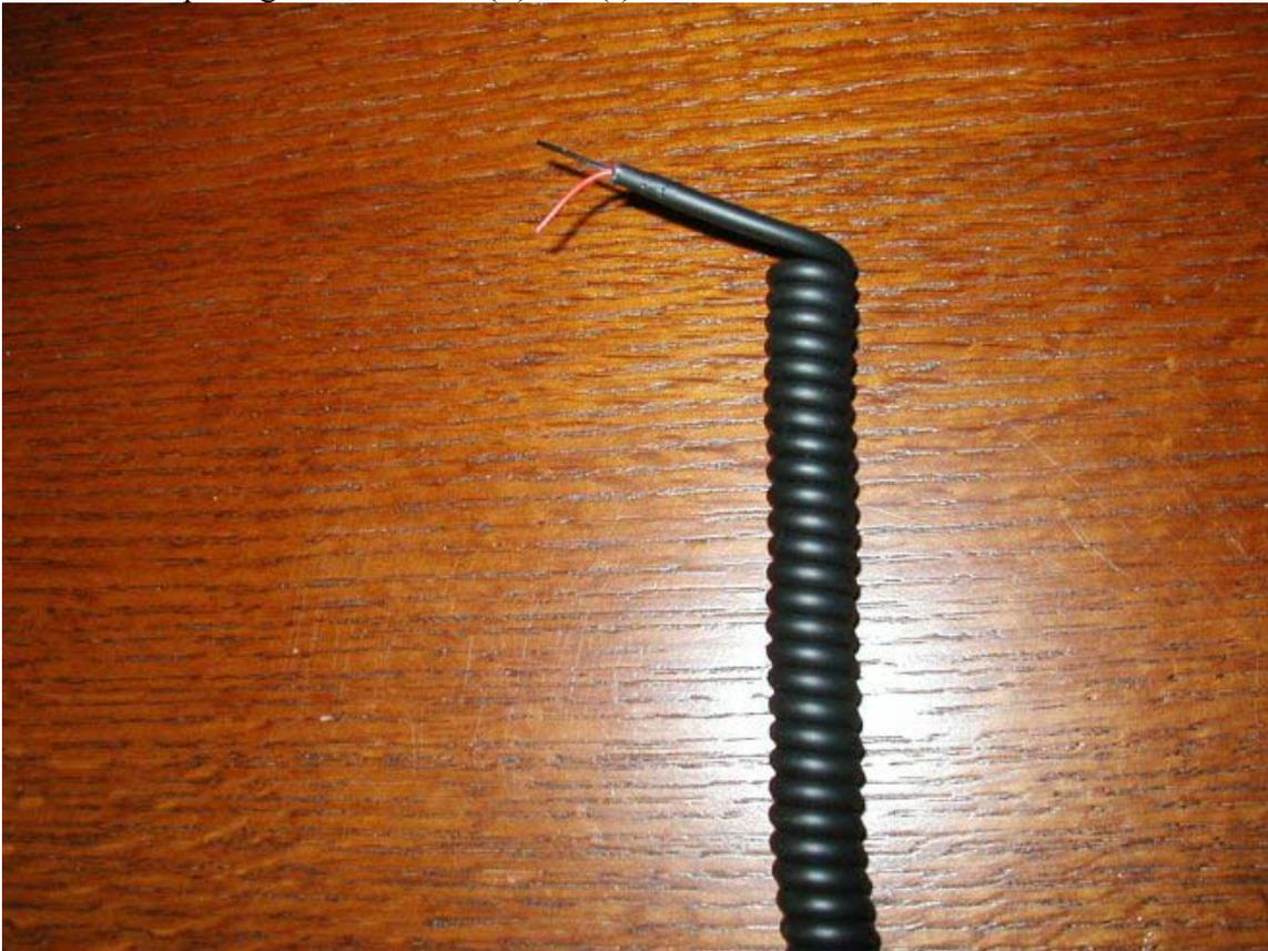
Step 5: Strip 1/2 and inch or so of insulation from the red and black voltage wires from both the hotsync adapter and the car charger ends. After you strip them, twist the loose ends tight (keeps in neat).
