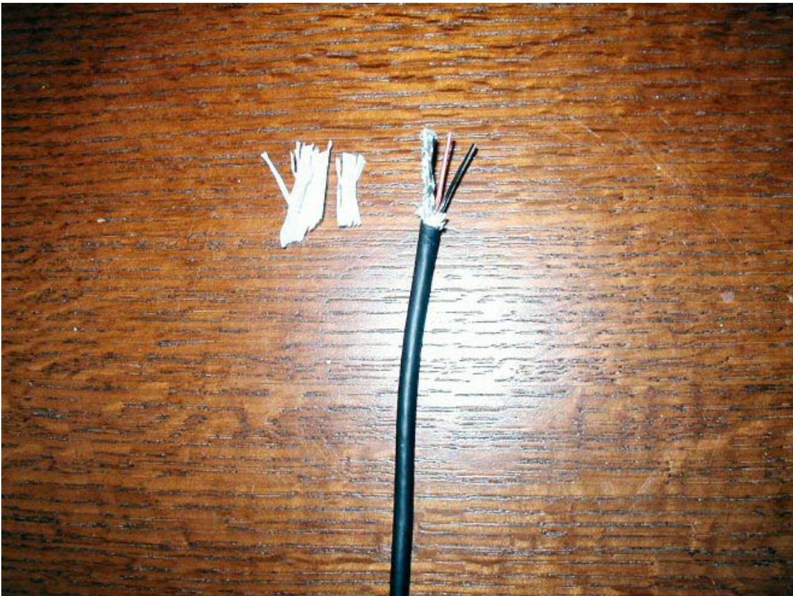
Step 3: Remove the wire mesh shield surrounding the USB cables. This exposes 4 little wires-- green and white for data, black for ground red for power (used for hotsync only, not connected to charger). Bend the tips and tape them over to prevent shorts (not sure if this would actually do anything but seems a prudent precaution).
